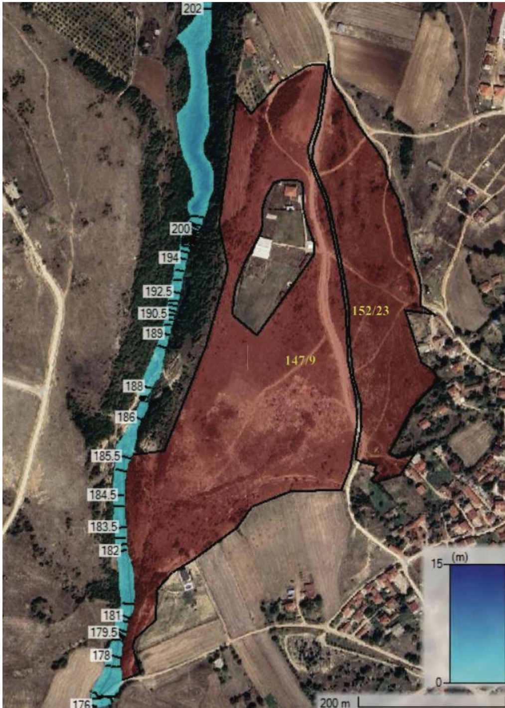
Figure 10: Overlay of the 500-Year Flood Analysis and the SPP Sub-project Area
